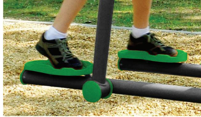
**UV resistant with high value of light fastness rotomolded or enjection polyethylene parts are used to form the structure on the grip, steps etc in fitness series. All parts are manufactured with double wall technique with the thickness between 4-6 mm.**
